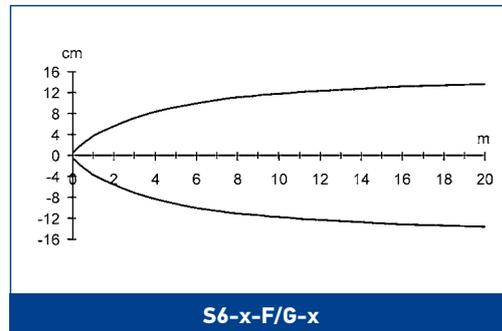
The detection diagrams indicate the typical operating distance with excess gain 1.
