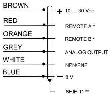
\* = Connect the unused REMOTE wires to 0 V.
