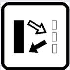
Luminescence sensors emit invisible ultraviolet light, which is reflected at a higher wavelength (minor energy) on the fluorescent and phosphorescent surface, shifting into the visible light spectrum.
