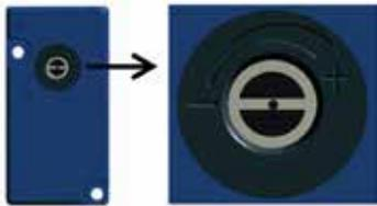
Emitter is equipped with a manual regulation which lets the user change the emission power by means of a screwdriver. The emission power reduction can be particularly useful to lower passive reflections when maximum operating distance it is not required.
