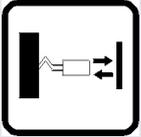
In photoelectric sensors with this optic function, both emitter and receiver are placed inside the same housing. These sensors work with weaker signals because the emitted light beam is reflected to the receiver by the object. As a consequence, the excess gain and the operating distance are reduced. However objects are detected without a prismatic reflector, making installations quick and easy.
