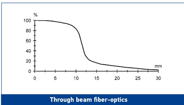
The detection diagrams indicate the typical operating distance.
