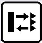
Both emitter and receiver are located inside the same housing for retro-reflective photoelectric sensors. Utilizing a prismatic reflector, the emitted light beam is reflected onto the receiver, detecting the object when it interrupts the light beam.
