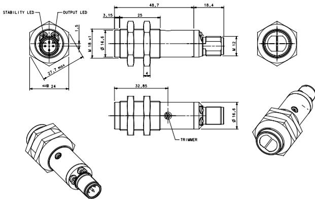
Through beam emitter - M12 connector version
