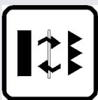
For the detection of transparent objects, such as PET bottles or Mylar sheets, a low-hysteresis polarized retroreflective model (which detects small signal differences) can be used.
