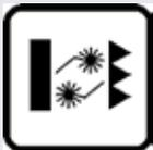
In polarized retroreflective sensors, the emitted light is polarized on a vertical plane through a polarization filter. The prismatic reflector rotates the light plane by 90°. A polarization filter placed on the receiver selects only the horizontal plane reflected by the prismatic reflector, ignoring the light reflected by other light sources. This technique guarantees a reliable signal reception, reaching significant distances-
