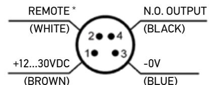
\* REMOTE INPUT (mod. S8..W, U, T50, T53), LIGHT / DARK INPUT (mod. S8..M53), DELAY (mod. S8..M Laser), TEST INPUT (mod. S8..G), ALARM OUTPUT (mod. S8..B, T51), NOT USED (mod. S8..C, M, F)
